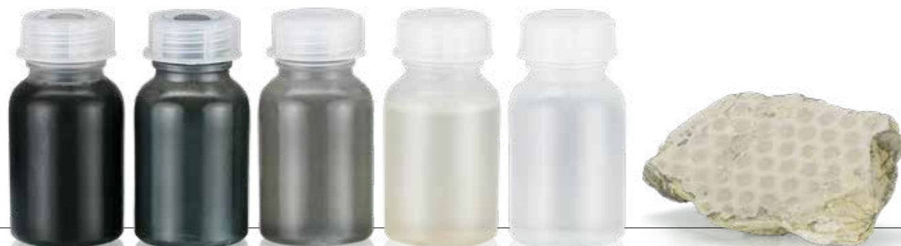
Water filtration samples from the treatment process, filterable solids are bound into filter cake.
