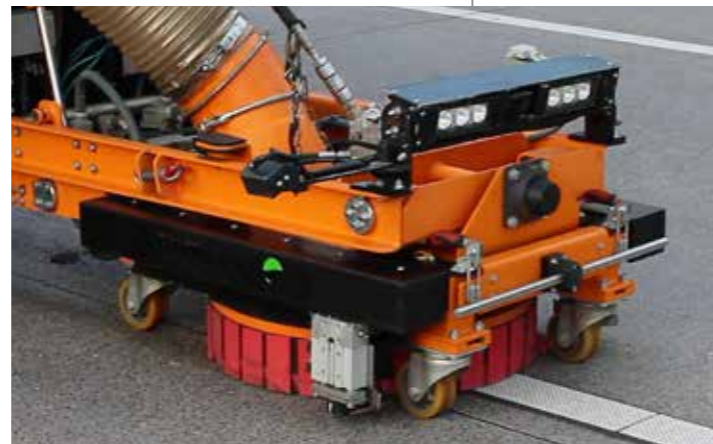
Joints on roads or airfields are dynamically covered over during the ongoing marking removal process.
